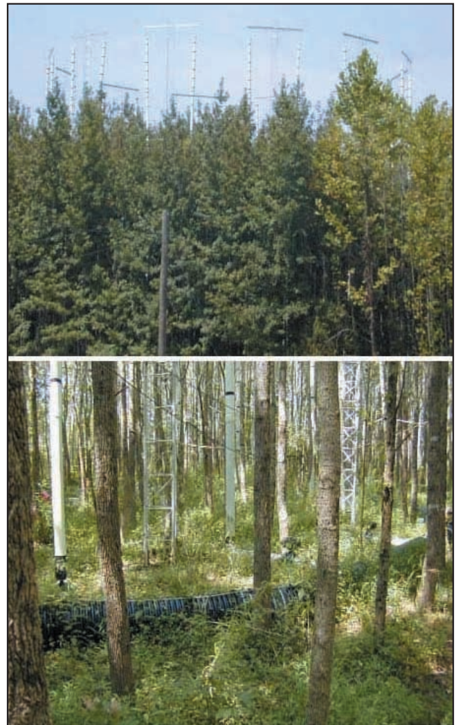
Figure 5. An experimental stand of sweetgum ( Liquidambar styraciflua ) trees at Oak Ridge National Laboratory, Oak Ridge, TN, exposed to elevated atmospheric CO 2 . (top) Twenty-four vertical vent pipes encircling each 25-m diameter plot emit CO 2 into the 15-m tree canopy to maintain canopy CO 2 at about 565 ppm. (bottom) The understory plant community within the sweetgum stand is dominated by Japanese honeysuckle ( Lonicera japonica ), a C 3 woody vine, and Japanese grass ( Microstegium vimineum ), a C 4 annual grass, both considered problematic plant invaders in the southeastern United States.
